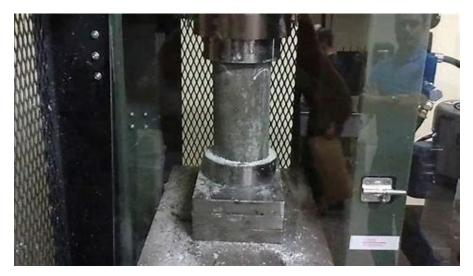
Cylinders used for acceptance of concrete should not be confused with field cured cylinders. Tests of field cured cylinders are used to evaluate whether the in-place concrete has been properly cured and protected, to estimate the early age strength in the structure for stripping of forms, post tensioning and/or to continue construction activity.
